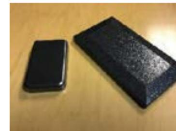
In their finishing area, they have the typical spray booth and a powder coating area. They have the technology to powder coat wood. They need to monitor the water content of the wood and calibrate the machine to work around humidity in the facility. Photo to the left shows powder coated wood.
