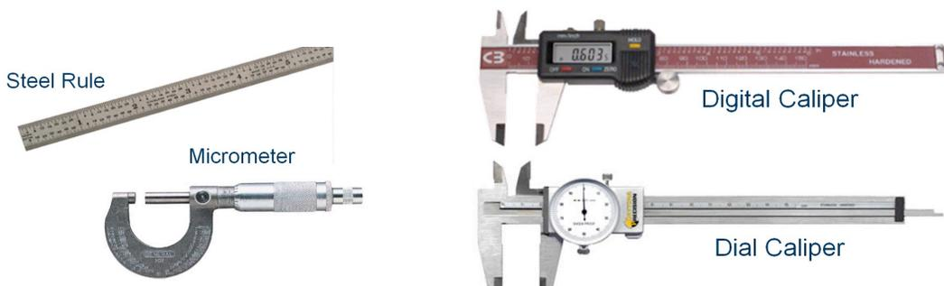
Teacher: We will be using a Dial Caliper to measure thickness, diameter and depth of ten objects.
