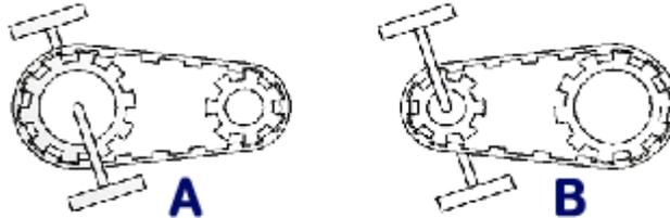
The gear train in which diagram provides more torque?   B
